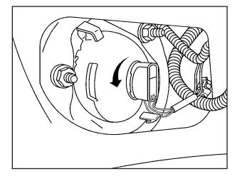
Remove the bulb socket by turning it counterclockwise.
